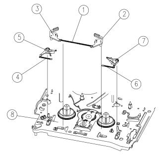
Fig.3-14 S/T MAIN & SUB BRAKES REMOVAL
